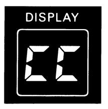
This flashing code tells you to check temperature controls and adjust them if necessary. (See directions on page 5.) Touch STATUS CHECK-RESET pad to erase code. If code reappears after 4 hours, call for service.
